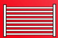
Steel rectangular hollow pickets either in 50mm x 10mm or 75mm x 16mm, and are horizontal for a modern look. Please note that this design is not suitable to use as a balustrade.
