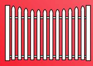
Steel rectangular hollow pickets either in 50mm x 10mm 75mm x 16mm, with shaped tops to resemble traditional wooden pickets. Pickets are longer on the edges and shorter in the middle to form a curve.
