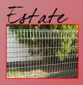
Traditional roll-top fencing panels. Manufactured from 5mm galvanised wire with veritical wires at 50mm centres and horizontal wires at 150mm centres. Standard panel length is 2400mm and in heights of 900mm and 1200mm
