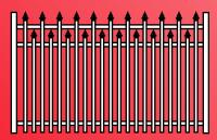
High low pickets with a choice of spears. Typically with the high pickets above the top rail and low pickets between the middle rail and top rail.
