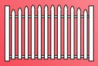
Steel rectangular hollow pickets either in 50mm x 10mm or 75mm x 16mm, with shaped tops to resemble traditional wooden pickets. Pickets are shorter at the ends and higher in the middle to form an arch.
